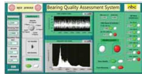
Bearing Quality Assessment System developed for NBC Bearing (NEI, Jaipur)
