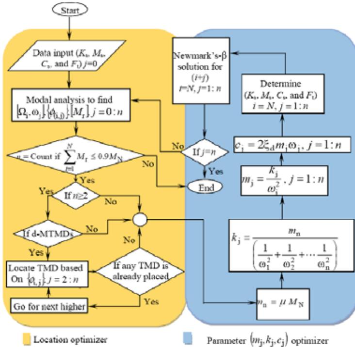
(a) Multi-Mode Dynamic Response Control using Spatially Distributed Multiple Tuned Mass Dampers.
