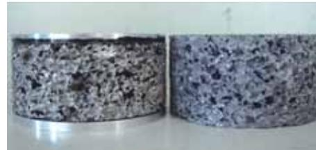
(a) Aluminum Syntactic Metallic Foam and Polymeric Foam Materials.
