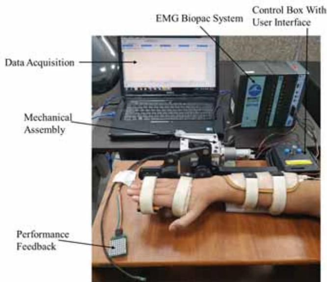
Figure: Set-up of the exoskeleton device for right hand with a patient.
