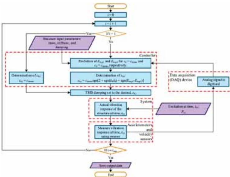
(b) Energy Based Predictive (EBP) Semi-Active Control Algorithm for Tuned Mass Dampers.
