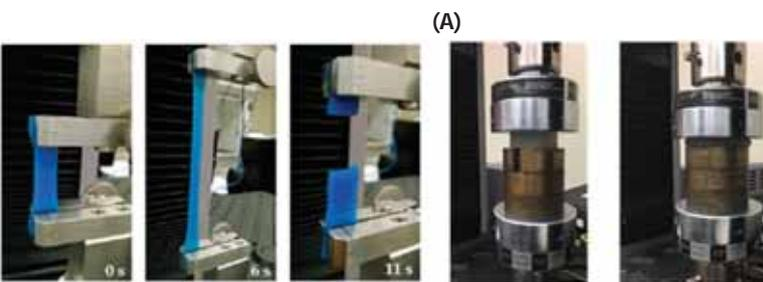
Figure 2: Mechanical testing of soft tissue surrogates: (a) Tensile and compression tests, (b) Comparison of true stress versus true stretch of surrogate compositions (FWFs) with natural tissue properties
